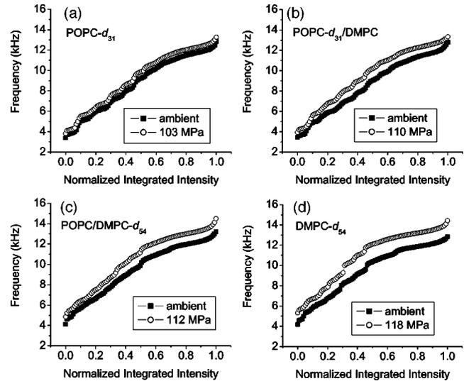
FIG. 7. Frequency vs normalized integrated intensity across the methylene region of the de-Paked spectra at ambient pressure (solid symbol) and  $\sim 110$  MPa (open symbol) for (a) POPC- $d_{31}$ , (b) POPC- $d_{31}$ /DMPC (1:1), (c) POPC/DMPC- $d_{54}$  (1:1), and (d) DMPC- $d_{54}$  at 45 °C.
