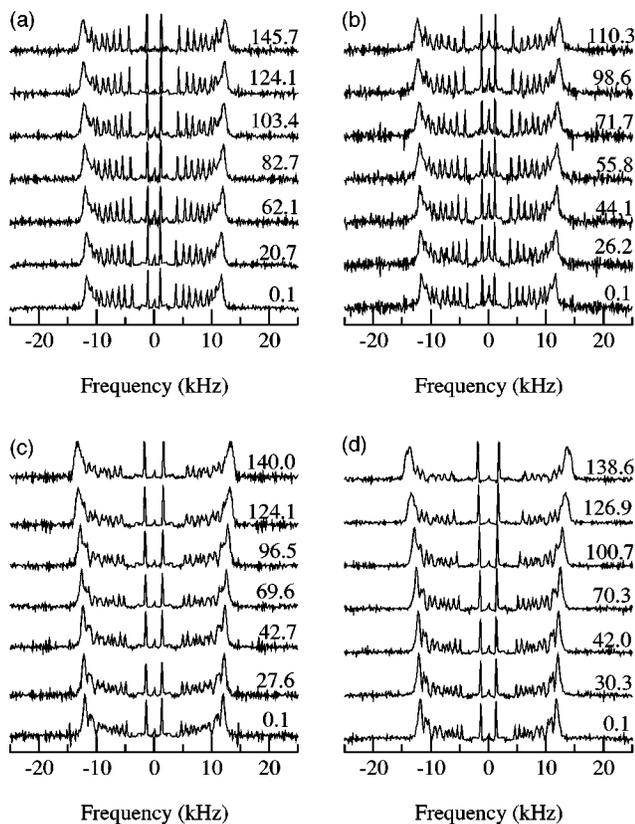
FIG. 2. Spectra corresponding to oriented samples obtained by de-Pake-ing of powder spectra for (a) POPC- $d_{31}$  (b) POPC- $d_{31}$ /DMPC (1:1), (c) POPC/DMPC- $d_{54}$  (1:1), and (d) DMPC- $d_{54}$  at 45 °C and selected pressures up to  $\sim 145$  Mpa. Spectra are labeled by pressure in MPa.
