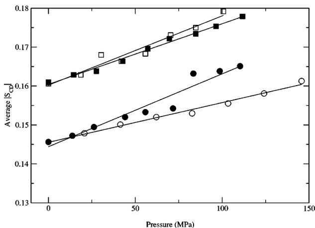
FIG. 3. Pressure dependence of average saturated chain orientational order for (○) POPC- $d_{31}$ , (●) POPC- $d_{31}$ /DMPC (1:1), (■) POPC/DMPC- $d_{54}$  (1:1), and (□) DMPC- $d_{54}$  at 45 °C.
